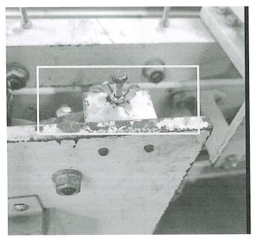
Wing nut installed in Semi-Auto 4 last April 20, 2022
